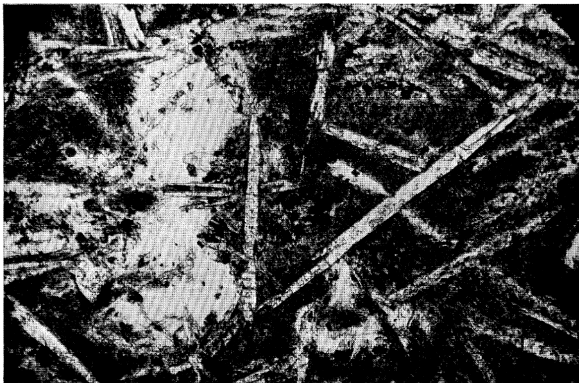
FIGURE 12. A splite pseudomorphing a variolitic basalt. This is the analysed specimen 4 of tables 2 and 3. Ordinary light; magn. \times 50 .
